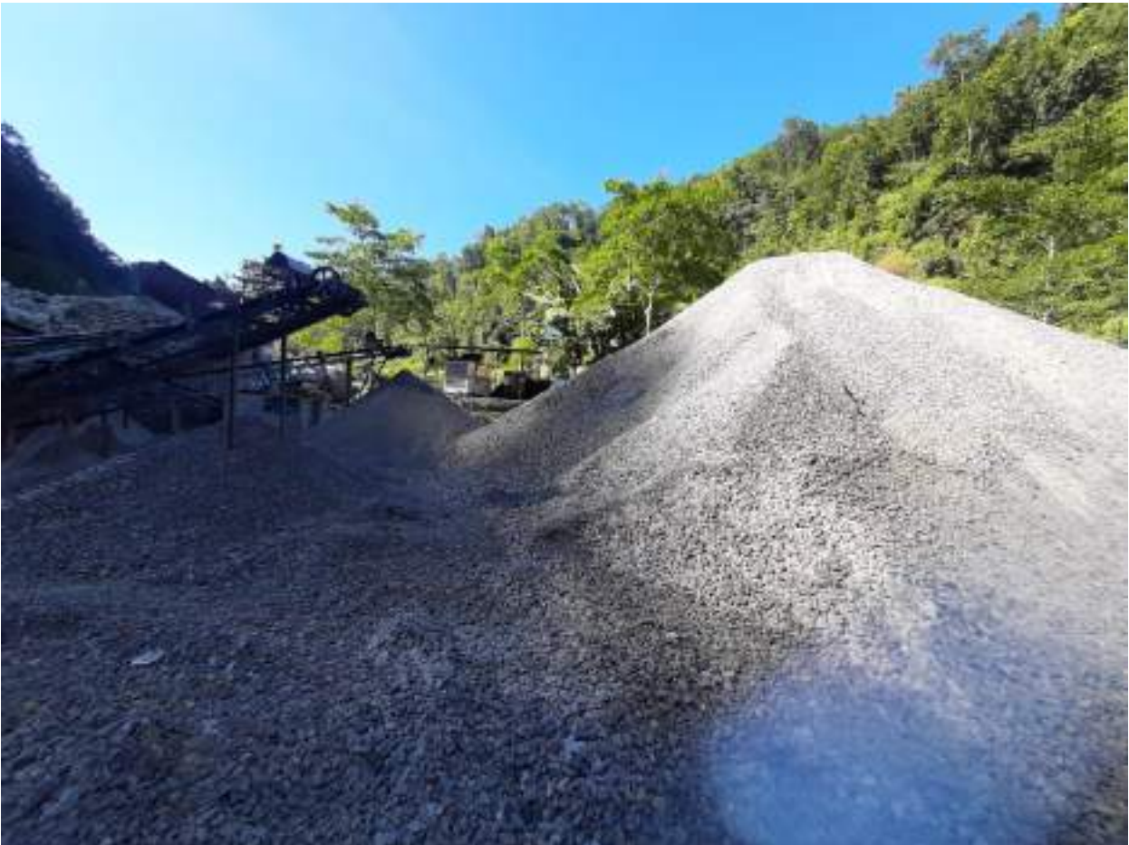
4-18: Aggregate produced by crusher at site
